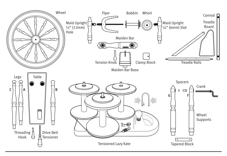
Join the two treadle rails with a 38mm ( $1\frac{1}{2}$ ") countersunk screw. Secure the treadle board to the treadle rails with four 32mm ( $1\frac{1}{4}$ ") countersunk screws.
