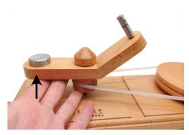
Step 4: Place the winding post onto the spindle, while keeping the spindle raised.
